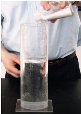
A cylinder filled with water and a little chalk dust is placed upon the overhead mask and has white light shining through it. The water in the cylinder will appear slightly ...
